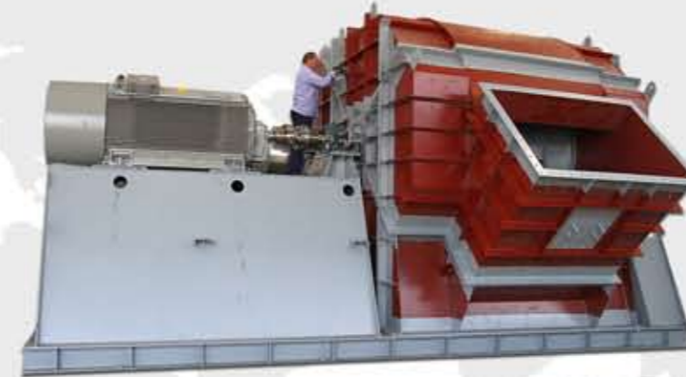
Induced Draft Fan
